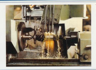
Cylindrical grinding is a process of grinding to include all outside grinding of round work even though the finished part is not always a true cylinder. The work may be, for instance, conical in shape or it may consist a special form grinding with the face of the wheel dressed to an irregular shape.
